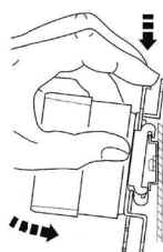
Fixing a contactor
